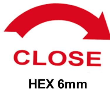
Figure 1: Example: A 6 mm Allen key is needed to close the OTV clockwise
